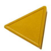
This is a a MT-CVD TIN coated functionally graded WC-Co carbide within ISO range P20-P45, for fine to medium machining of steels
