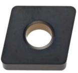
It is a submicron grade without cubical carbides with low content of cobalt. This grade is for general purpose applications for all groups of work material except P. This grade is suitable for small up to medium chip cross section with steady cutting conditions.
