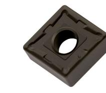
This is a MT-CVD coated functionally graded WC-Co carbide within ISO range P20-P45, for fine to heavy machining of steels
