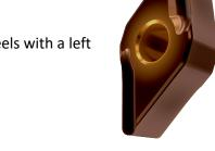
This grade is a PVD coated fine grained WC-Co carbide within ISO ranges P25-P40 and M20-M35, for medium to heavy machining of steels and stainless-steels with a left handed turning tool
