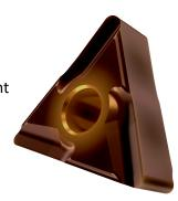
This grade is a PVD coated fine grained WC-Co carbide within ISO ranges P25-P40 and M20-M35, for medium to heavy machining of steels and stainless-steels with a right handed turning tool
