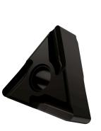
This grade is a MT-CVD coated functionally graded WC-Co carbide within ISO ranges P15-P35 and M10-M30, for medium to heavy machining of steels and stainless-steels with a right handed turning tool
