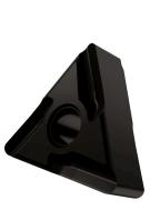
This grade is a MT-CVD coated functionally graded WC-Co carbide within ISO ranges P15-P35 and M10-M30, for medium to heavy machining of steels and stainless-steels with a left handed turning tool
