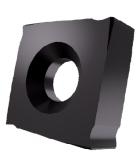
This is a TIALN PVD coated fine grained WC-Co carbide within ISO-grade range P25-P50 for machining of steel with disc mills 938
