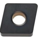
Grade with very high resistance to chemical wear; suitable for finishing operations using high cutting speeds. With its high abrasion resistance, it is also suitable for productive K01 – K15, machining of hardened and treated materials
