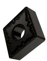
This is a MT-CVD coated functionally graded WC-Co carbide within ISO range P05-P25, for fine to medium machining of steels
